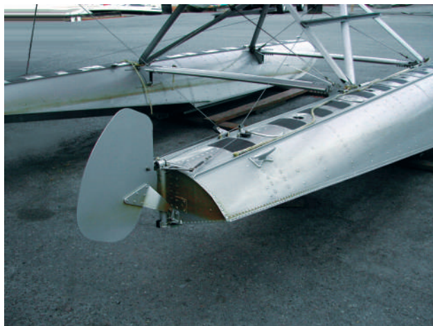
Figure 4-4. Inspect the water rudders, cables, springs, and pulleys for proper operation.
